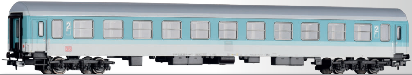
Reisezugwagen 2. Klasse Bom 280.1, Bauart Halberstadt, der DB AG 2nd class passenger coach Bom 280.1, type Halberstadt, of the DB AG
