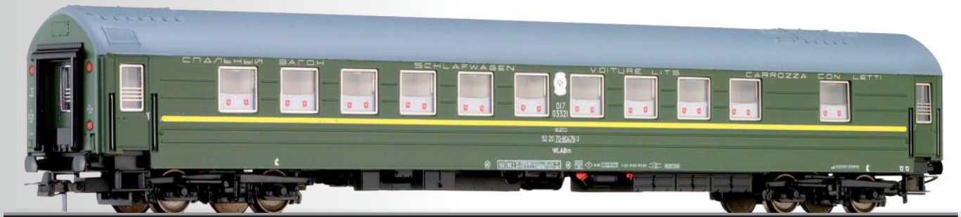
Schlafwagen 1./2. Klasse, Typ Y, der SZD 1st/2nd class sleeping coach, type Y, of the SZD
