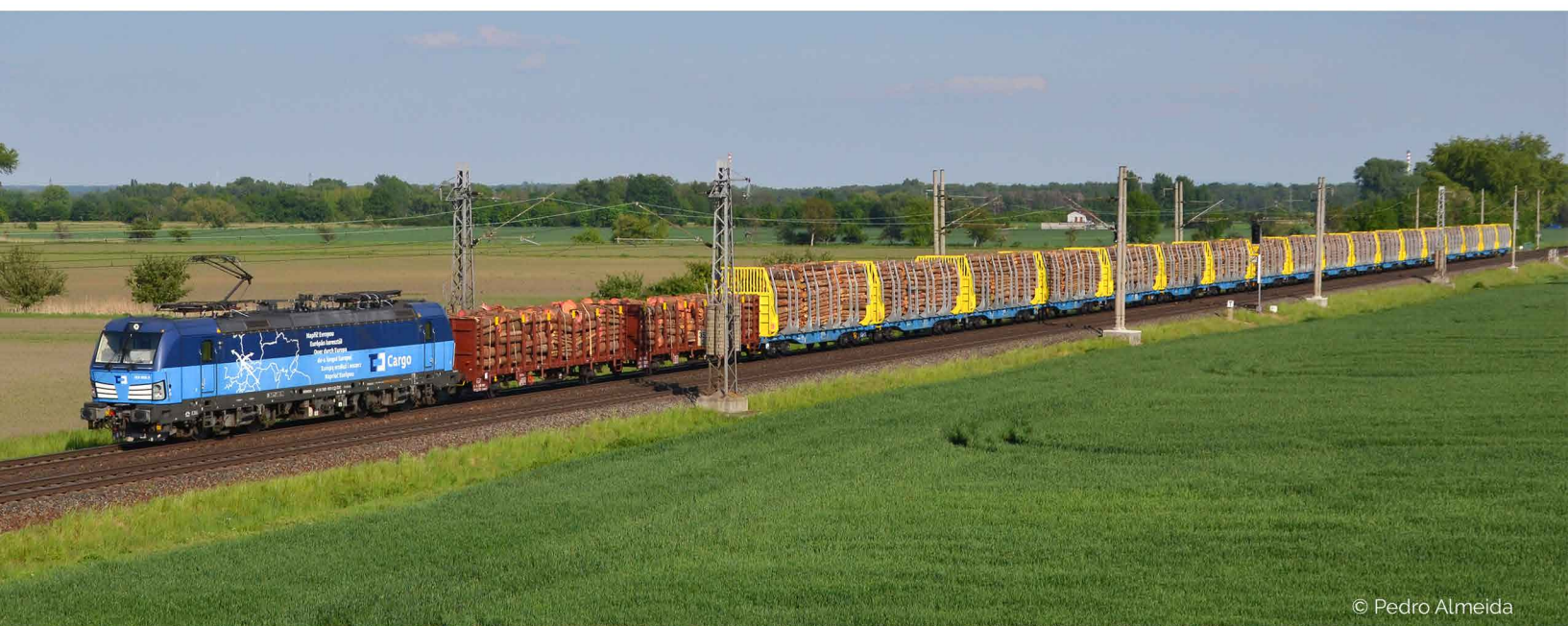
S657009 CD Cargo articulated double timber transport wagon Sggmrrs | CD Cargo Doppel Holztransportwagen Sggmrrs - A-IF 35 81 4657 009-0
