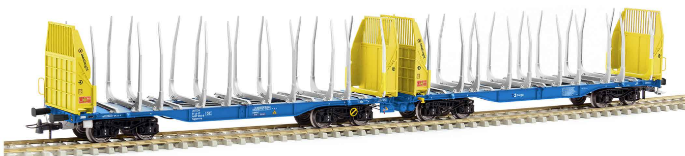
S657111 CD Cargo articulated double timber transport wagon Sggmrrs | CD Cargo Doppel Holztransportwagen Sggmrrs - A-IF 35 81 4657 010-8
