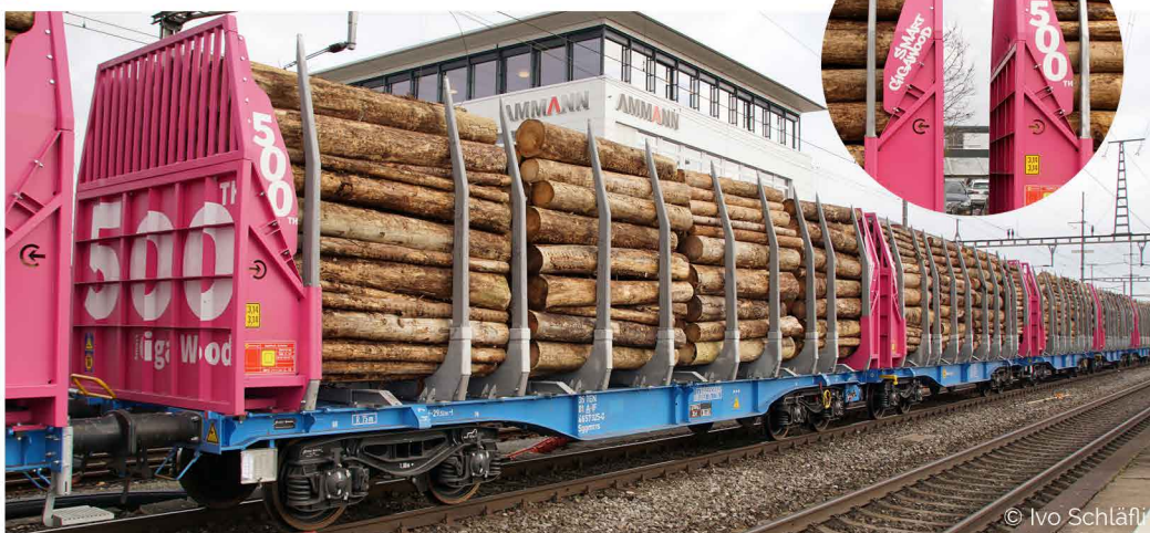
S657325 Innofreight articulated double timber transport wagon Sggmrrs | Innofreight Doppel Holztransportwagen Sggmrrs - A-IF 35 81 4657 325-0 "500TH Smart GigaWood"
