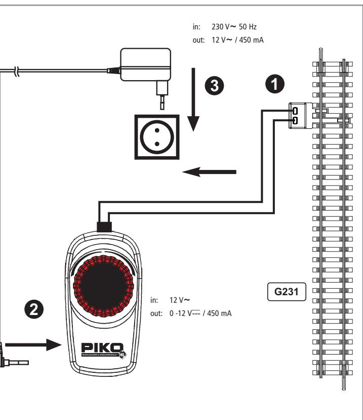
such as switch machines, signals and lamps with this mains adapter or speed controller. The speed controller does not possess a separate alternating current exit. The technical details and data are all on the base plate of the units.
