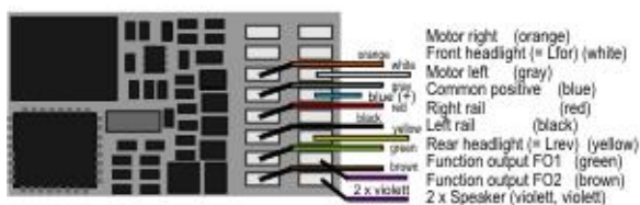
MX648 Top View with wires
