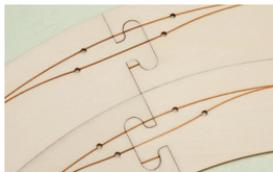
**Curves:** Vehicles swing out, just as in real traffic, i.e. if traffic enters a curve the wire is routed outward. The curve sections can be used from both sides so that the same section can be used for right and left curves.
