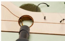
**Drill holes:** The break-out and the offset for branches are prefabricated in the contact wire routing so that it only needs to be inserted and secured. Holes are predrilled in any wise location along the contact wire routing for inserting sensors.
