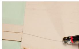
**Groove cutter:** Now preferably mark the desired driving path and cut the groove for the contact wire with a Groove Cutter (161669). Implementing your ideas doesn't get any easier and quicker. This allows you to build any design you would like yet benefit from FALLER Laser-Street.
