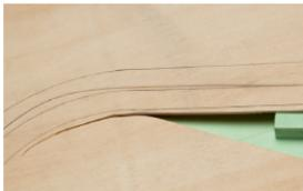
**Planning:** Mark the roadway by outlining it on the plywood and perform a test run to ensure the roadway is uniform. To do so lay out the wire, affix it with an adhesive strip and test the route with a vehicle.
