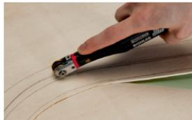
**Cutting:** The Groove Cutter (161669) is ideal for installing the special contact wire. This small machine features a slitting cutter which is guided along the marked path. Cutting the right groove height and width allows for optimal contact wire installation.
