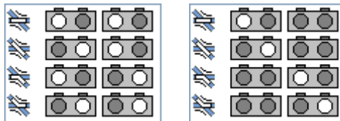
Diagram 71: Decoder Configurations for a double slip turnout
