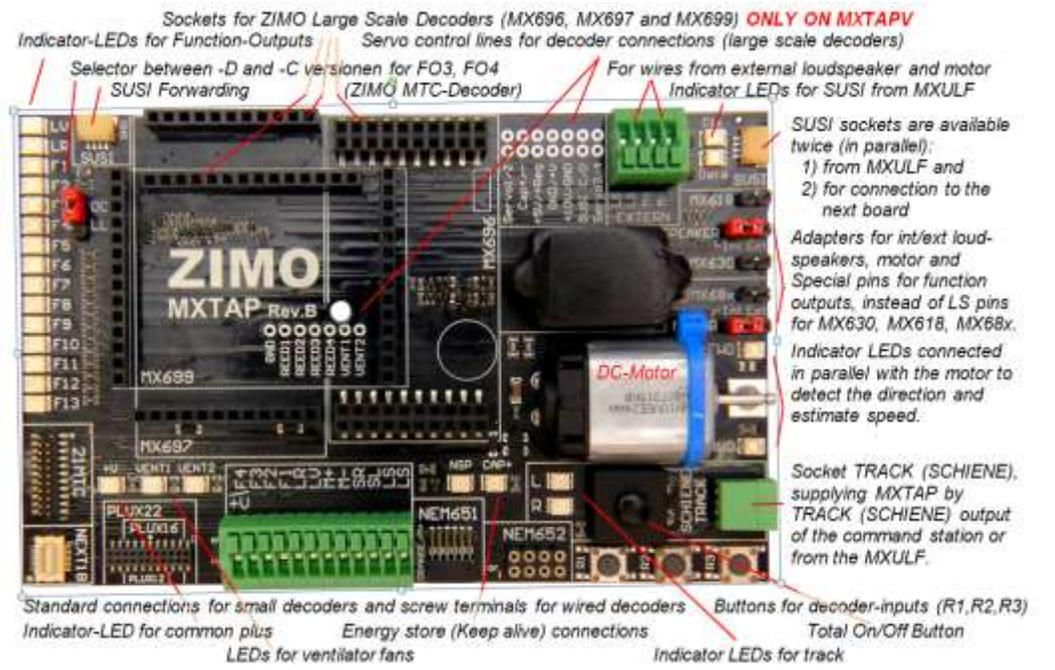
The **MXTAPS** (or **MXTAPV**) is connected to the output "Schiene" of the **MXULF** via the double clamp "SCHIENE", and to a track output of a ZIMO central command station or another digital command station. No additional supply is necessary.
