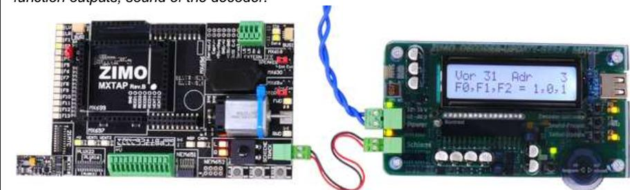
*MXTAPV* with decoder *MX648R* (8-pole *NEM652* interface, speaker not on interface, therefore, wires on clamps), connected to *MXULFA*:
