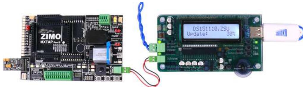
**MXTAPV** (not **MXTAPS**) with connected large-scale decoder **MX696**, connected to **MXULFA**; on the **MXULFA** **sound loading** was just started (according to the display), the sound project is loaded **from a flash drive**.
