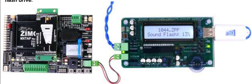
**MXTAPV** with decoder **MX645P22** (PluX22), connected to **MXULFA**: additionally **SUSI** cable between **MXULFA** and **MXTAPV**, for **faster sound loading via SUSI**, **MXULFA** in this case is controlled **by computer** (usually software **ZSP** - ZIMO Sound Programmer; USB cable to the computer; on the display information to communication between PC and **MXULFA**).
