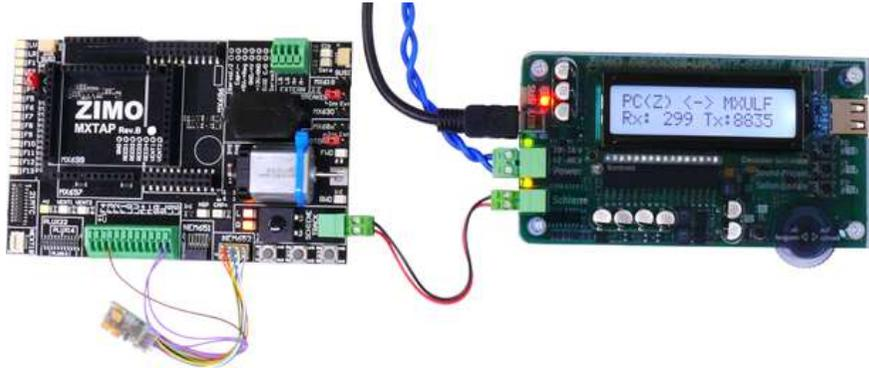
**ATTENTION:** To load sound into large-scale sound decoders, the SUSI interface ("SUSI" plug) on the decoder itself has to be used; it is NOT provided on the pin connectors of the decoder and therefore also NOT on the SUSI pins of the MXTAPV!
