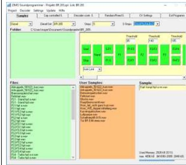
▲ **ZSP** (creation of sound projects, decoder updating, sound loading): in the picture above you see the display during the software update of a sound decoder MX645; MXULF is recognized as MX31ZL (because the MXULF behaves the same).
