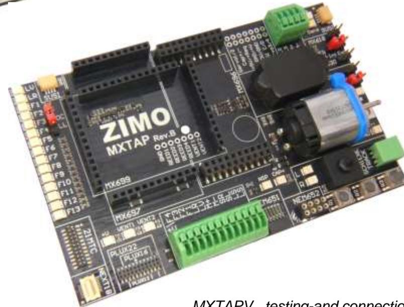
MXTAPV testing-and connection board
