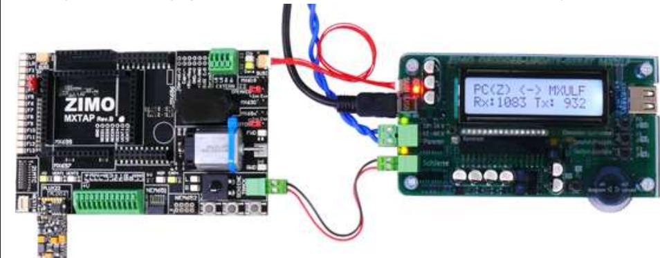
**MXTAPV** with decoder **MX648N18** (Next), connected to **MXULFA**: Via operating elements and display of the **MXULFA**, **test operation** is active, i.e. tests motor control, function outputs, sound of the decoder.
